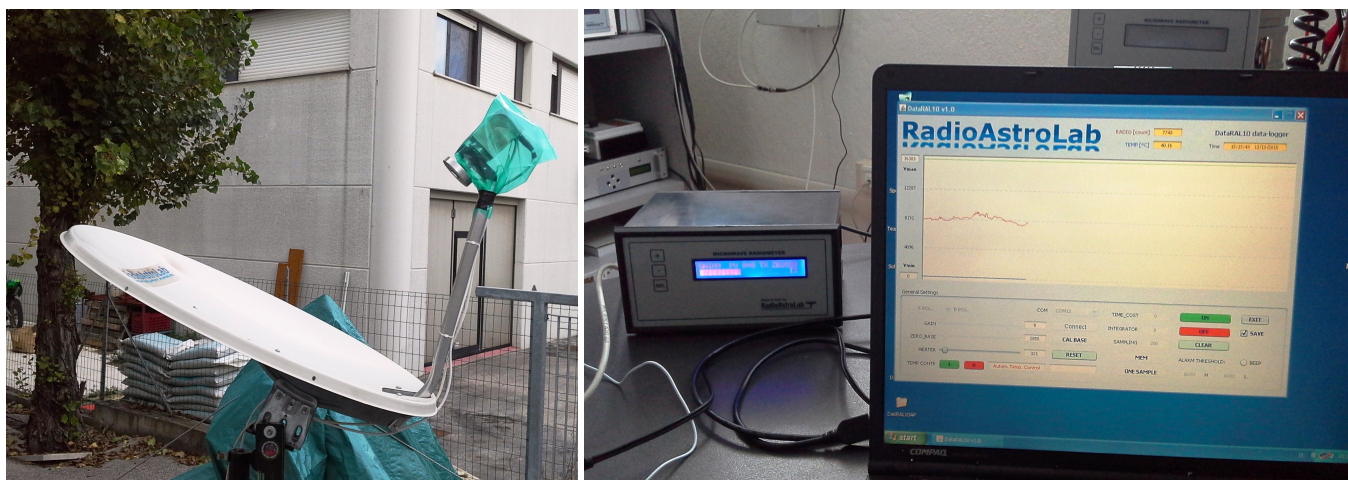
Pic. 2: The radio telescope used in the experiment: you can see the antenna (a common offset parabola for TV-SAT 10-12 GHz of 70 cm) equipped with the external unit RAL10_LNB and the receiver RAL10.
