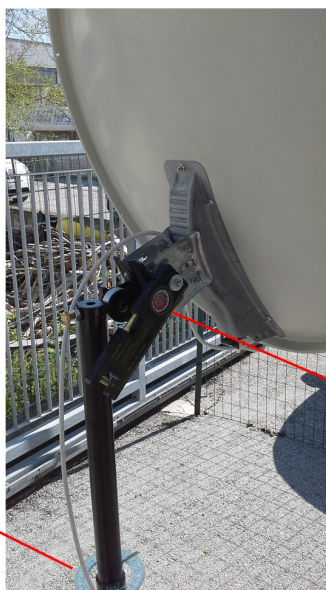
Pic. 3: Orientation system of the antenna: it is a simple amateur realization where the pointing is realized manually by controlling the elevation and displacement in azimuth of the beam of reception so that it is coincident with the future position of the Moon, at the given instant of the fixed day.
