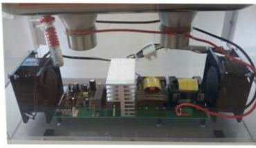
An example of the application of our technology: we have set up a demo that illustrates the technology of an ultrasonic cleaning system. You can see our RAL151 electronic generator, the ventilation system, the tank containing the cleaning liquid with the piezoelectric transducers applied on the bottom.
