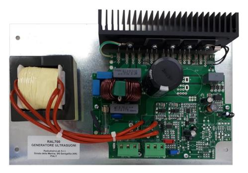
Modular power unit suitable for driving piezoelectric transducer arrays in industrial ultrasonic cleaning applications. Fully programmable and remotely controllable by means of a RS485 serial communication line.
